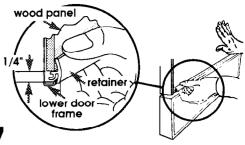
Insert retainer over lower edge of door frame while holding wood door panel up.
